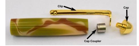
11. Start the assembly process by pressing the cap coupler completely into the top of the upper barrel using a pen press. Slide the clip over the cap screw and then twist the cap into the upper barrel.
